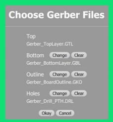
After pressing "Okay" the file should be shown on the preview. If needed use the "Placement" tool to adjust the location on the material.
