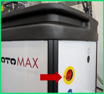
You can check if the machine is turned on by taking a look at the light inside the machine.
