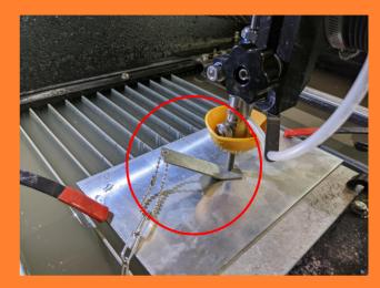
Bend the orange split guard to flip it over. Then move it down so it touches the surface.
