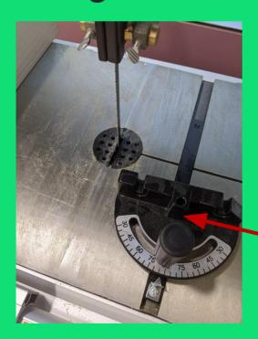
The push guide can be used to cut parts flat perpendicular to saw.
